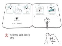
5. Add 6 drops of the Sample Treatment Solution to well A. Then rotate the swab for 2 rounds, each direction in the buffer.
